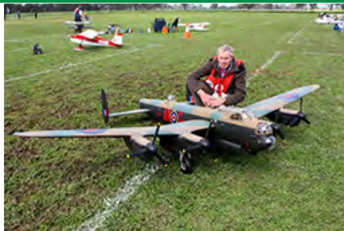
Ron Clark WRCS (NSW) Scratchbuilt Avro Lancaster 134" W/S 4 x Saito 21cc 4/stroke petrol engines
