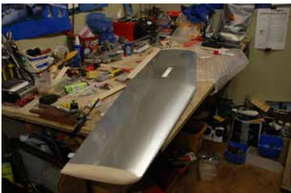
Balsa sheeted foam wing ready to move onto the next phase.
