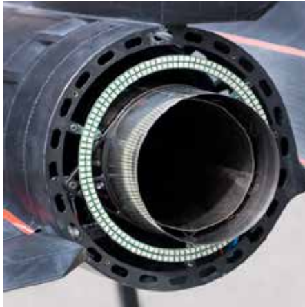
LED rings imitate the afterburners.
