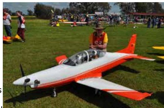
Ross Smith (Lithgow Club) and his 3rd scale PC21 Turbo Prop. Heavy duty gearbox connect to a Wren 44 turbine.
