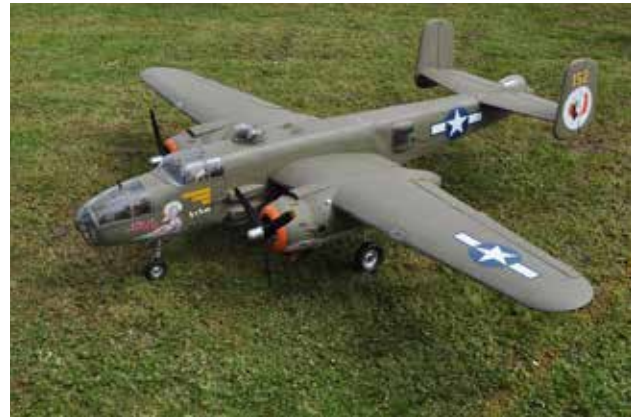
Ron Clark (WRCS NSW) with his B25 Mitchell. This is a ARF kit, Ron has extensively modified the kit and has excellent detail. Two 26 cc MVVS. 14 kg and 97" wingspan.
