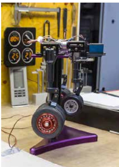
Product of hobby: All components for the undercarriage test rig as well as the mounted undercarriage were made using the machining centre
