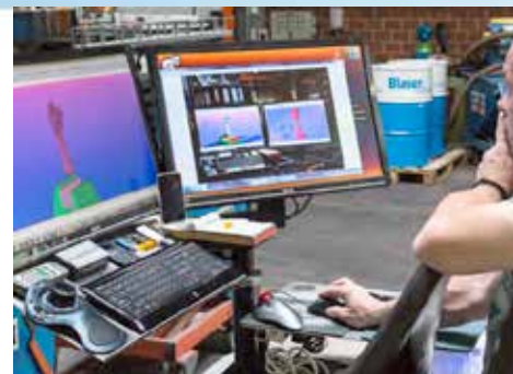
CAD system showing the strut support of the SR-71 main undercarriage on the screen.
