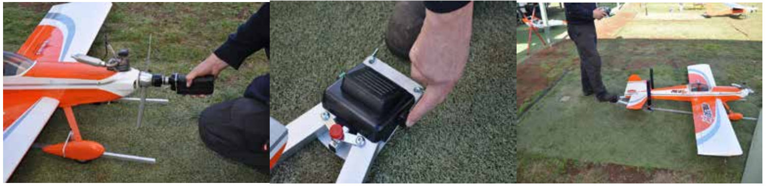
(Left) Starting is simple and look, one hand only... (Centre) Arming the foot trigger. This stops any accidental release from the restraint. (Right) Once all checks are complete, the pilot takes up his position, TX in hand and ready to release. Total control.
