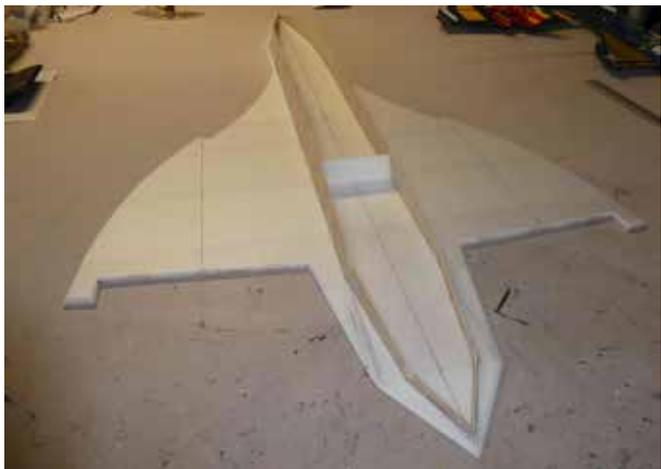
*Float hull in making.*
