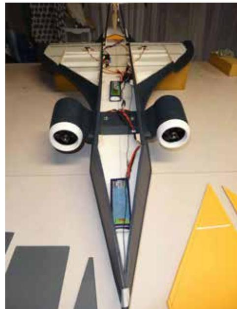
*Preliminary centre of gravity battery position checks.*
