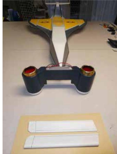
*Balsa laminated Elevon tabs ready for paint after water proofing.*
