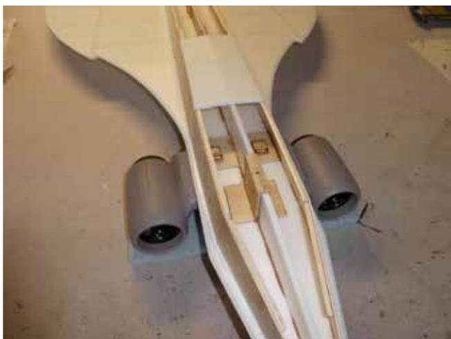
*Belly float hull ready for sealing off, after the nose gear and removable EDF power system installation.*
